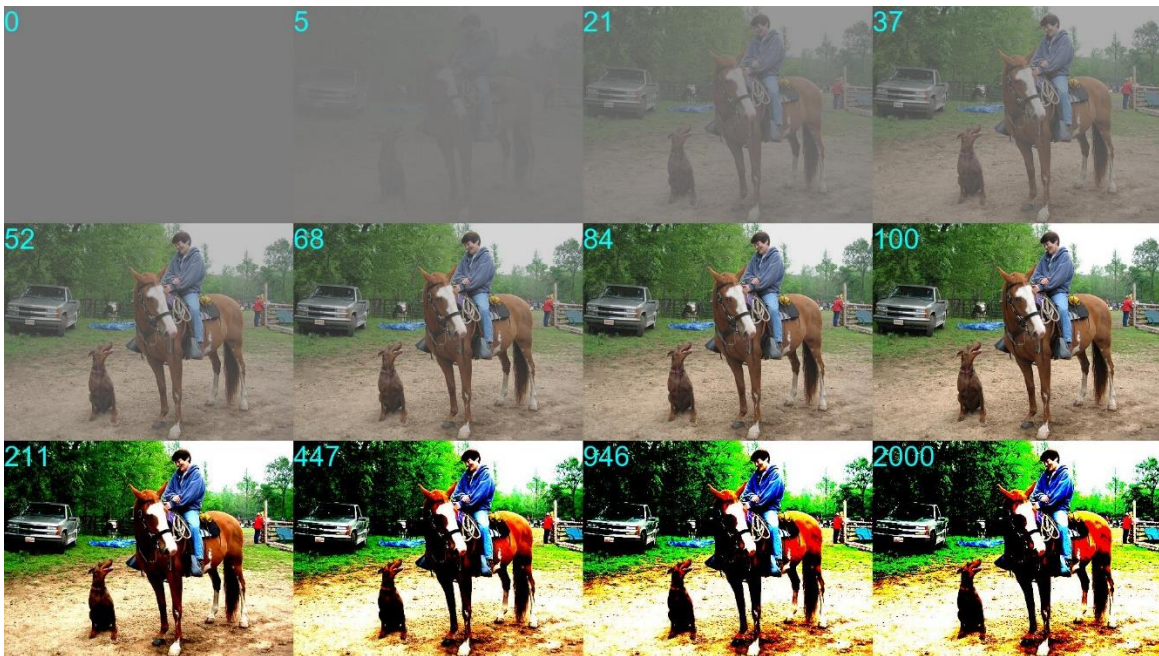
Figure 3.4 Example image displaying the various levels of contrast, indicated in the top left in cyan as a percentage. Contrast levels ranging from 0% (all gray) to 2000% (heavily contrasted), including 100% (untransformed).
