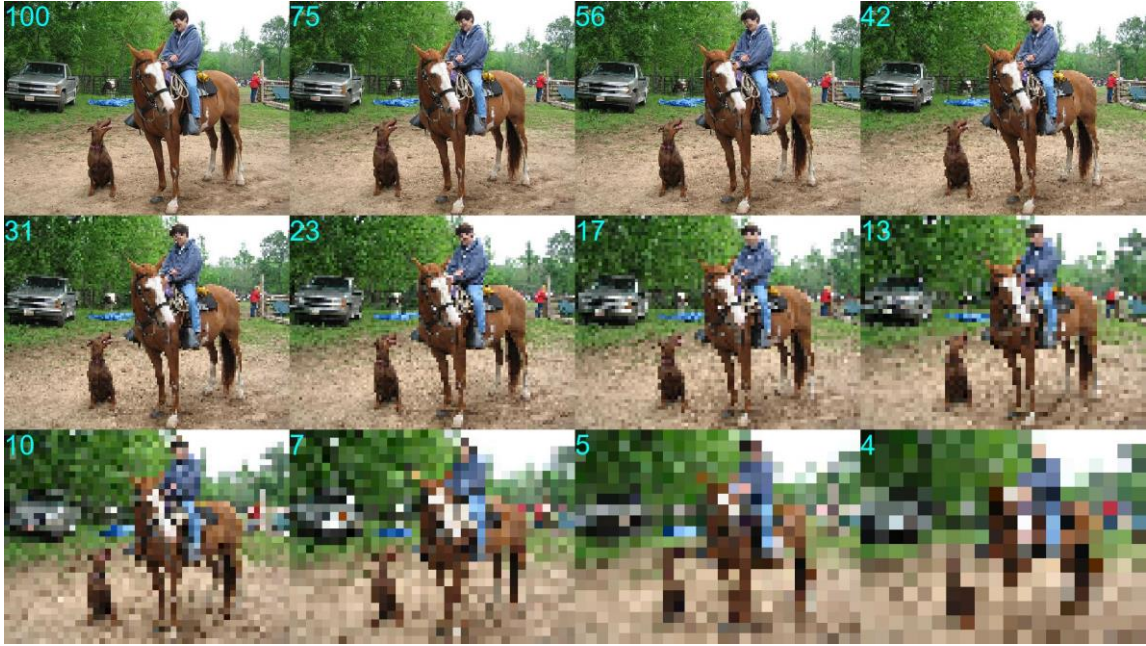
Figure 3.6 Example image displaying the various levels of image resizing, indicated in the top left in cyan as a percentage. Sizes ranging from 100% (untransformed) to 4% (pixelated). Resizing replicates pixelation by reducing the image by a given percentage of the original image size using the nearest neighbor filter, then upscaling the image to the original size.
