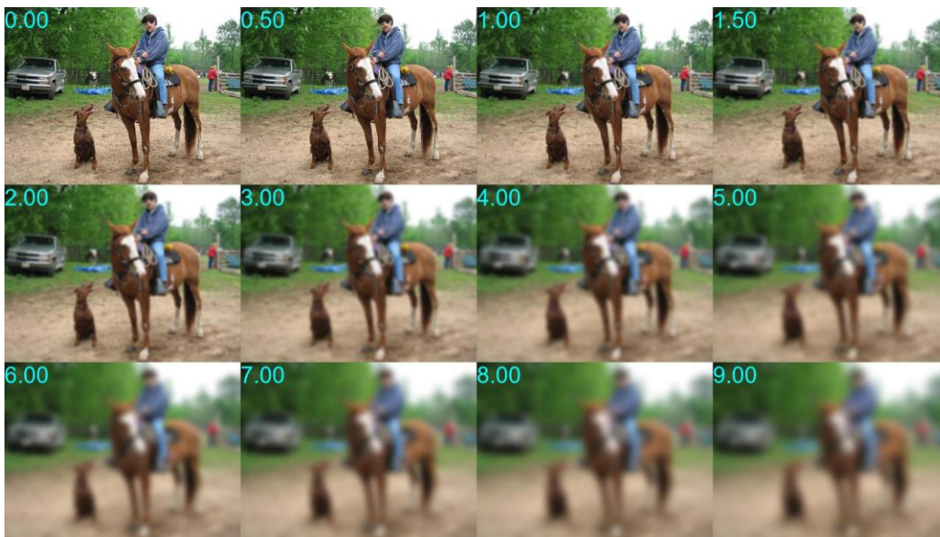
Figure 3.5 Example image displaying the various radii of Gaussian blur, indicated in the top left in cyan. Gaussian blur with radii ranging from 0 (untransformed) to 9 pixels (heavily blurred).
