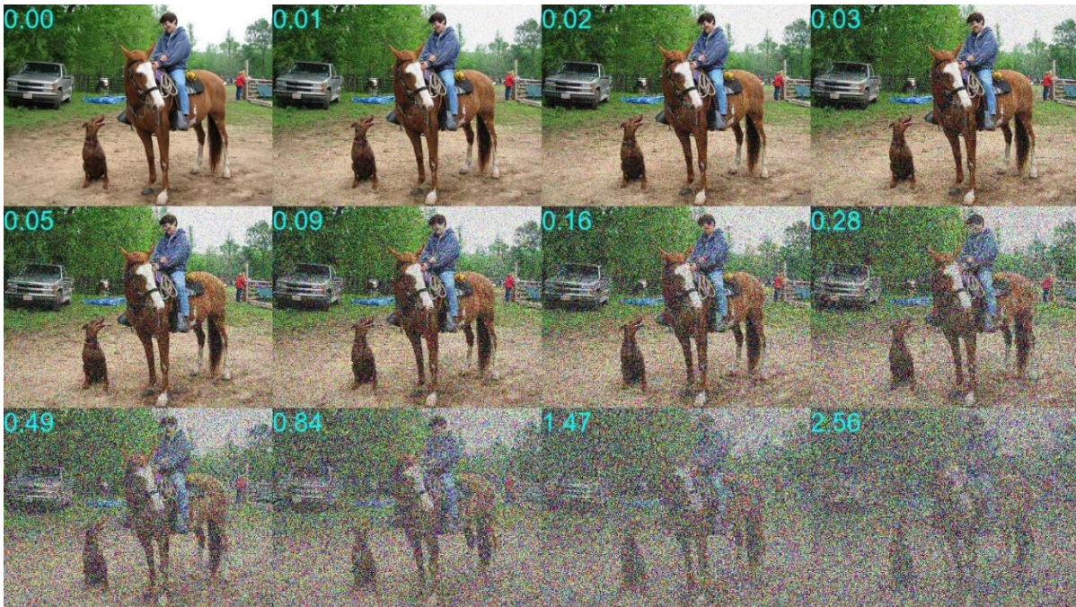
Figure 3.8 Example image displaying the various levels of Gaussian noise, indicated in the top left in cyan as the variance. Gaussian noise with variance ranging from 0 (untransformed) to 2.56 (very noisy).
