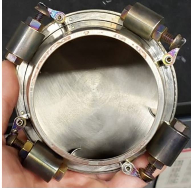
Figure 3.10: Tumbler with conical shape, having curved fins inside and four tapping weights around to shake powders inside.
