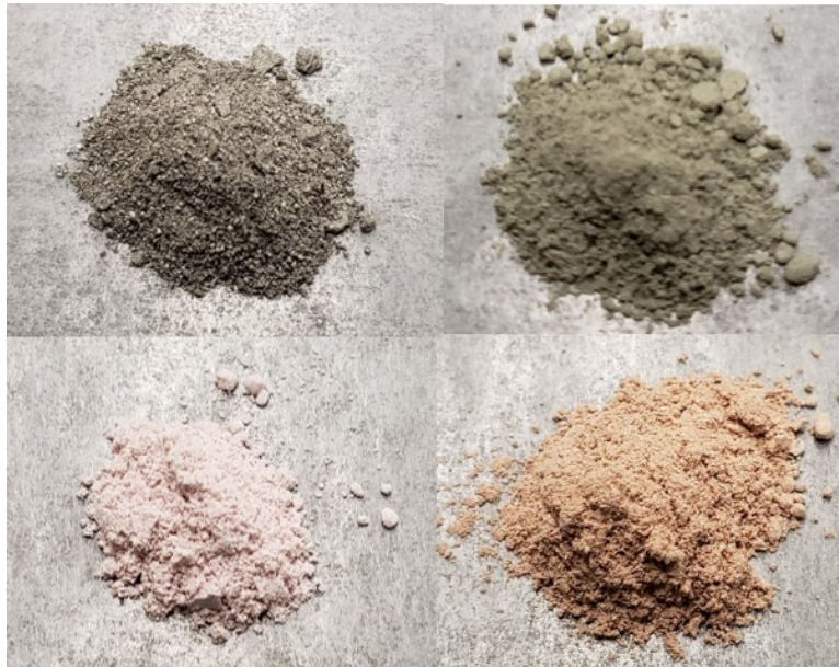
Figure 4.5: Cu/MgO powdered materials showing changes in coloration from deposition up to the highest post-deposition heat-treatment temperature. Top left: Cu/MgO right after deposition. Top right: Cu/MgO after heat-treatment at 500 °C (tapping devices in use). Bottom left: Cu/MgO after heat-treatment at 950 °C (tapping devices not in use). Bottom right: Cu/MgO after heat-treatment at 950 °C (tapping devices in use). Cu/MgO shows a black/gray color after deposition, and heat-treatment changes its color into shades of green (500 °C) and eventually pink/red (950 °C).
