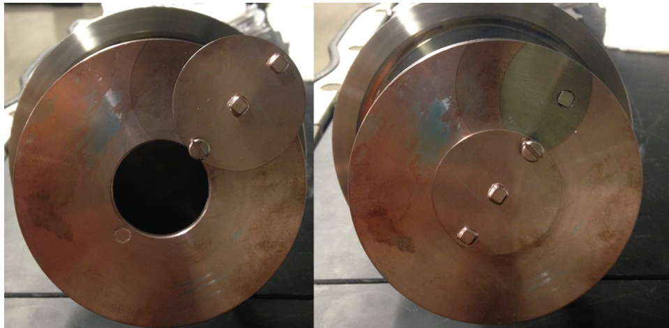
Figure 3.9: First version of the SS tumbler with cylindrical body. Here it is shown with the cover with lid described in the text ( left: open lid; right: closed lid ).
