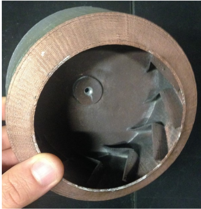
Figure 3.8: The first version of the tumbler (3D-printed).
