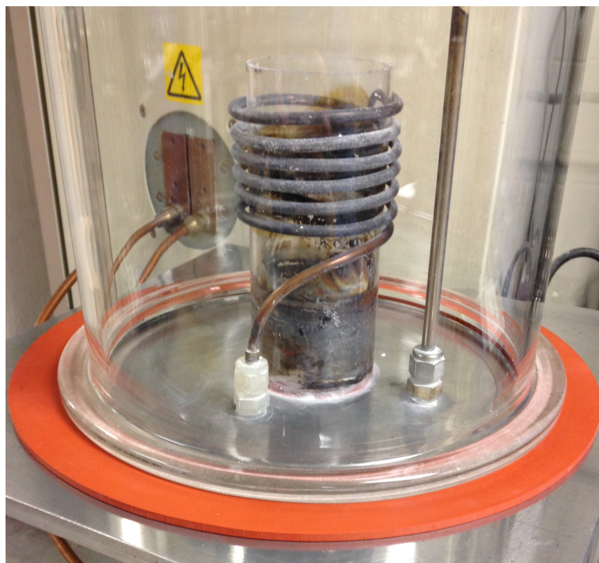
Figure 3.13: The induction furnace-based apparatus for the MO synthesis described in the text.
