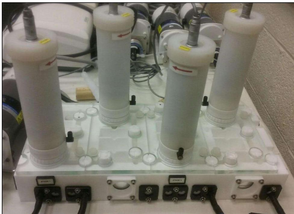
Figure 3A: 4-Stage UX 1.1 Mixer-Settler Used (Only 1 Stage Employed for Study)
