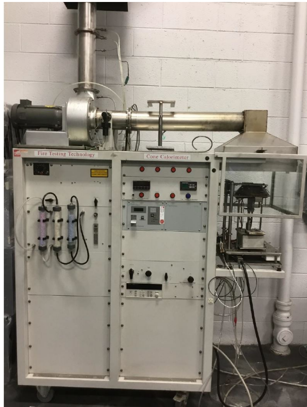
Figure 3.13: Image of the Fire Testing Technology Cone Calorimeter used for testing.
