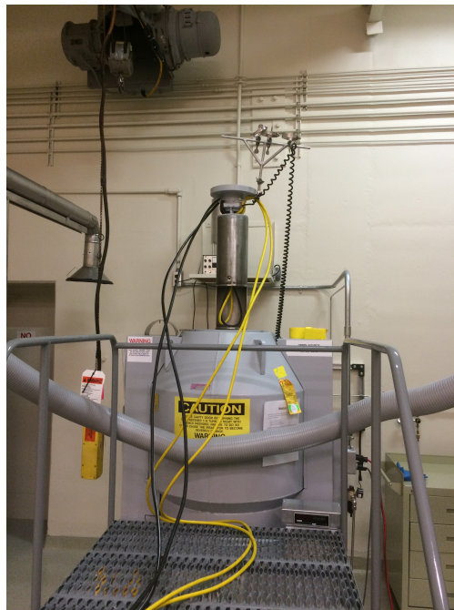
Figure 3.7: The Colbalt 60 source irradiation vessel that was used to irradiate the cable samples (image shown is of the Rockbestos Firewall III XLPE cable being irradiated).
