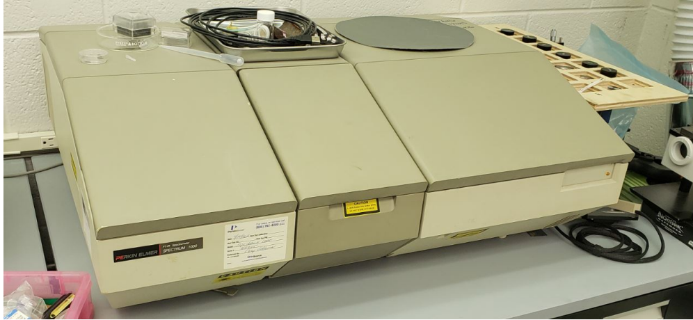
Figure 3.10: Image of a Perkin Elmer Spectrum 1000 Fourier-Transform Infrared Spectroscopy (FTIR) used for testing.
