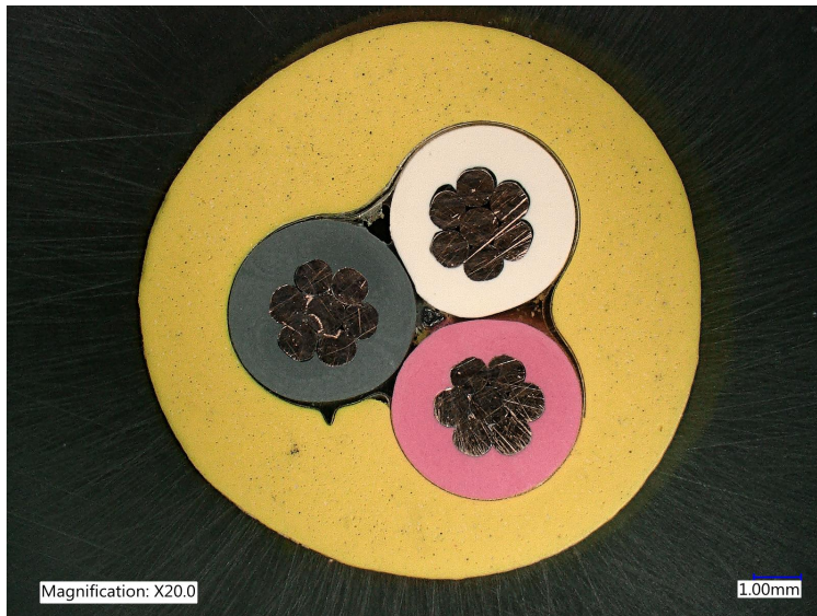
Figure 3.2: Cross sectional microscope image of Unaged Rockbestos Firewall III XLPE insulated cable.
