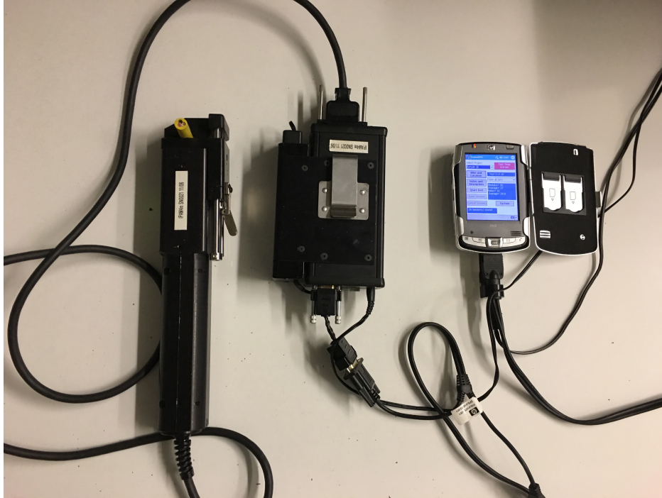
Figure 3.8: Indenter polymer aging monitor used to test elasticity of cable.
