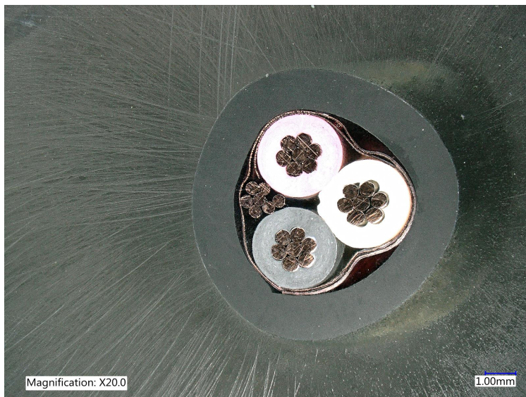
Figure 3.3: Cross sectional microscope image of Unaged ULTROL 60+ XLPE insulated cable.
