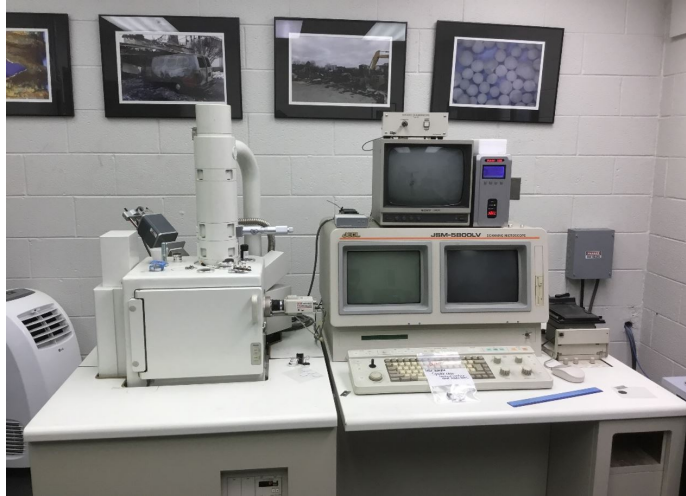
Figure 3.9: Image of Scanning Electron Microscope (JEOL 5800LV) used for testing.
