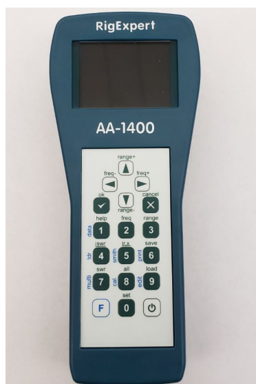
Figure 3.16: RigExpert AA-1400 antenna analyzer used for reactance measurements of cable samples.
