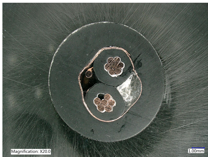
Figure 3.4: Cross sectional microscope image of Unaged Boston Insulated Wire (BIW) EPR insulated cable.
