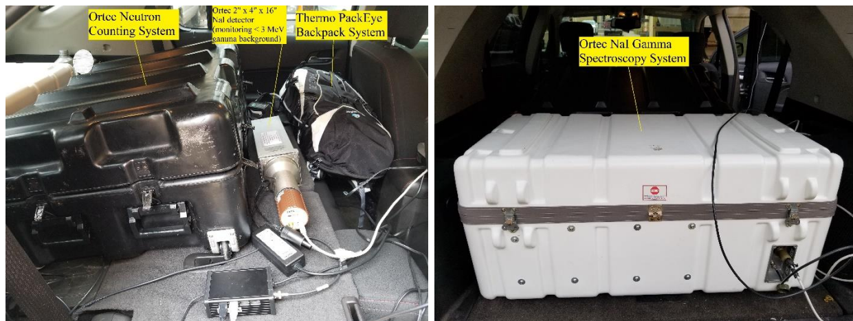
Figure 4. Photos displaying the detector systems' placements when mounted in an SUV-type vehicle for these measurements looking into the vehicle from the rear passenger side door (left) and the trunk (right).
