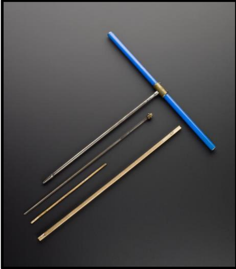
An example of a tree corer, that was used to gather the tree core samples in ALT properties.
