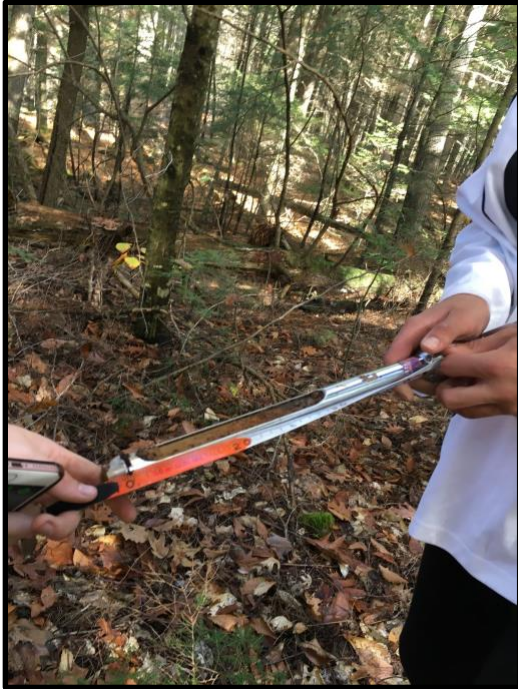
Photo to the left shows the sampled soil in the sampler being measured to the correct depth for volume purposes later on in the calculations. As mentioned above, 5 cm was measured here.
