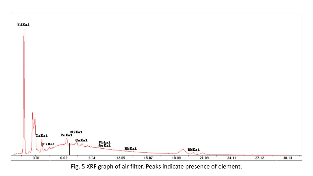
XRF analysis of 5 filters resulted in different heights of peaks, suggesting variable elemental composition of the particulate matter. XRF analysis only allows for a qualitative assessment and further analysis using ICP-OES is required to determine
