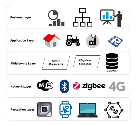
Figure 2.3: Five-layer Architecture of IoT
