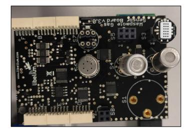
Figure 4.9: Waspmote Gases Board
