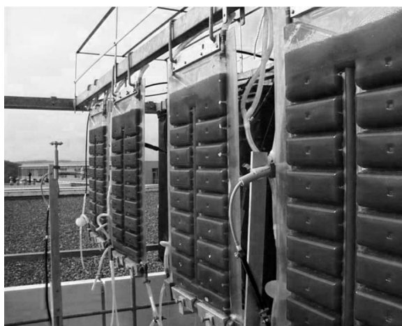
Fig. 3: The Airlift plate reactor of the firm subitec
