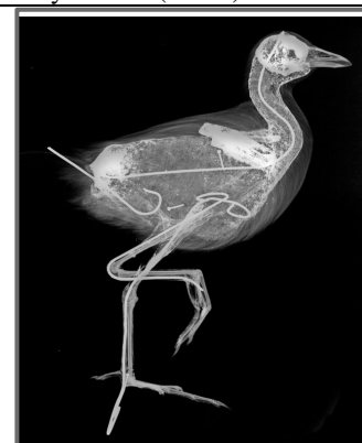
Figure 25: Taxidermy bird showing pockets of heavy metal pesticide residue (white clumps).
