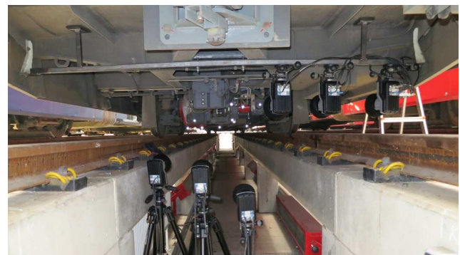
Fig. 9. The distribution of the Qualisys system six cameras.
