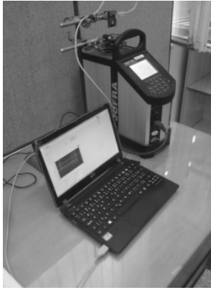
Fig. 5. Calibration - assembly of measuring system during calibration.
