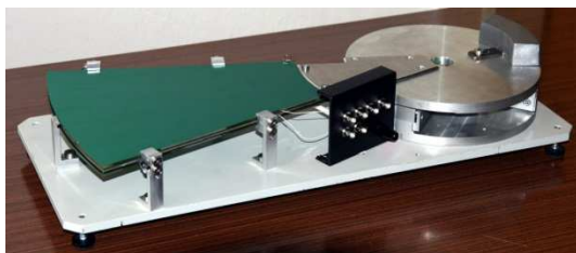
Fig. 11. Capacitive sensor of the angle of rotation
