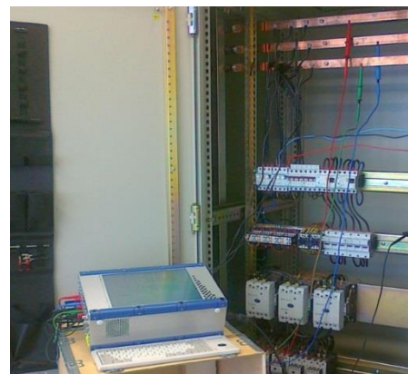
Fig. 41. Measurement of time waveforms and harmonic analysis in the laboratory down scaled model.
