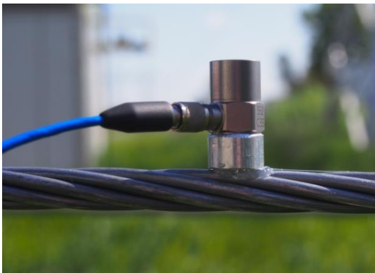
Fig. 5. Piezoelectric accelerometer attached on the conductor.
