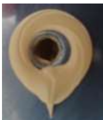
Fig. 9. Result of paste application along the circular path.
