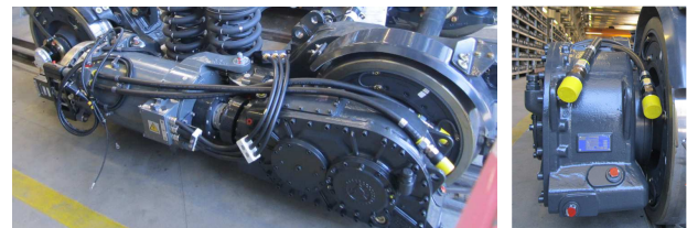
Fig.13. Concept of the traction drive in not pivoting trams bogie SKODA.
