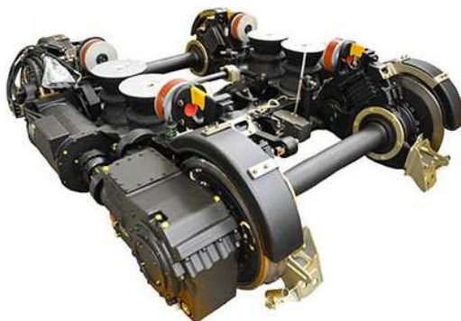
Fig.11. Concept of the traction drive in partly pivoting bogie Flexx Urban 3000 [Bombardier].
