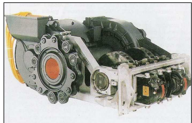
Fig.21. Full sprung wheelset drive HBA of the locomotive Taurus [Siemens].
