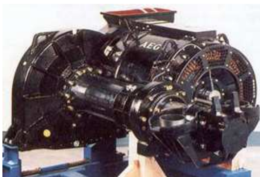
Fig.17. Design study of a modern wheelset drive concept with "paw motor" [ AEG ].
