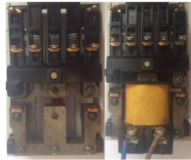
Fig. 13. Used electrically controlled switcher.
