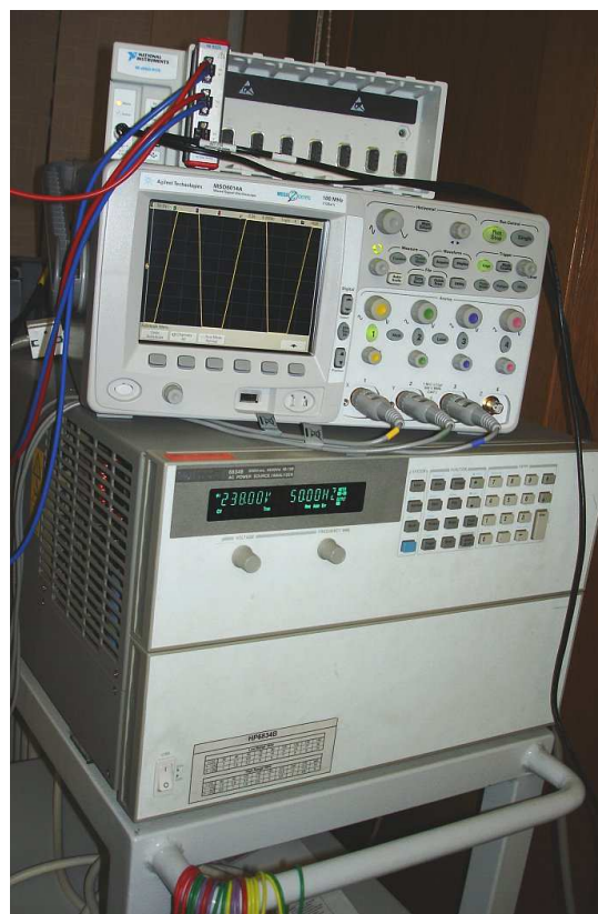
Fig. 1. Programmable power source HP6834B, AGILENT oscilloscope, National Instruments cDAQ chassis with NI9225 module
