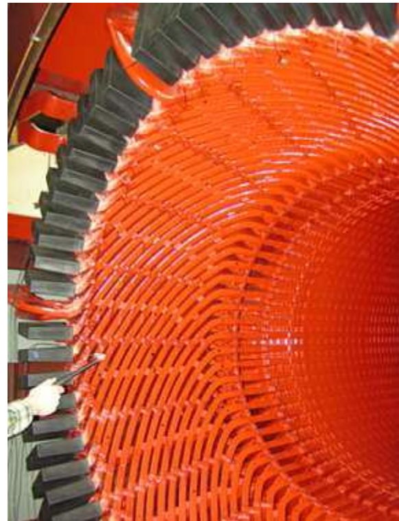
Fig. 9a. Modal analysis measured at the real endwinding.
