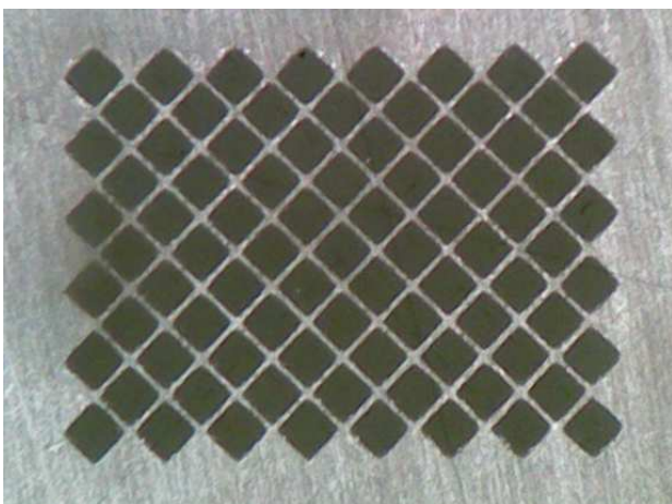
Fig. 3. EDM grid with 83 apertures 0.4 \times 0.4 \text{ mm}^2 and struts width 60 \mu\text{m} in 0.16 \text{ mm} thick molybdenum sheet [12].
