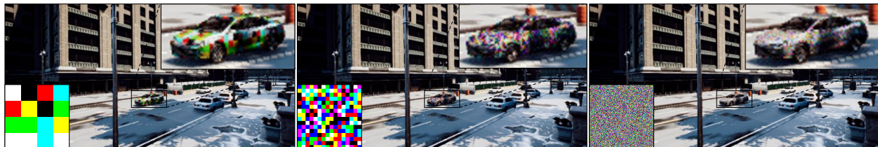
Figure 5.9: Visualization of three random camouflages of resolutions 4 \times 4 , 16 \times 16 , and 256 \times 256 , respectively, as well as the resulting images by the same camera.
