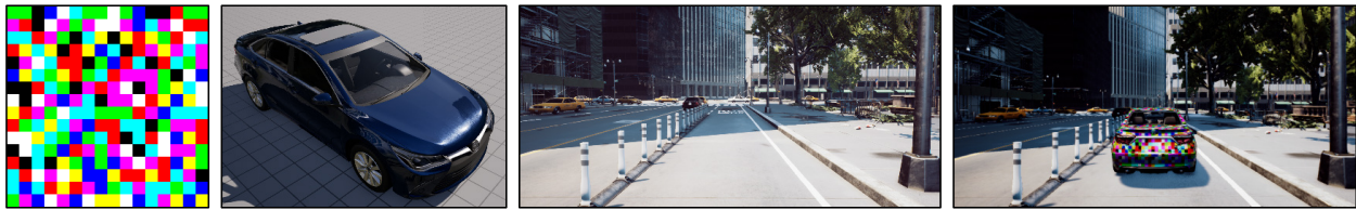
Figure 5.2: Example procedure of a transformation t . From left to right: a 16 \times 16 camouflage, a high-fidelity vehicle, a location in our simulated environment, and an image due to this transformation over the camouflage.
