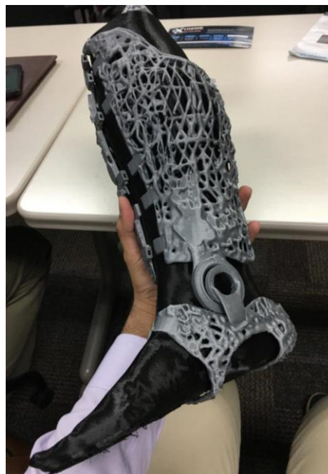
Figure 41. ML optimized cast provided by Stratasys
