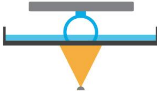
Figure 31. Diagram of bottom-up SLA machine
