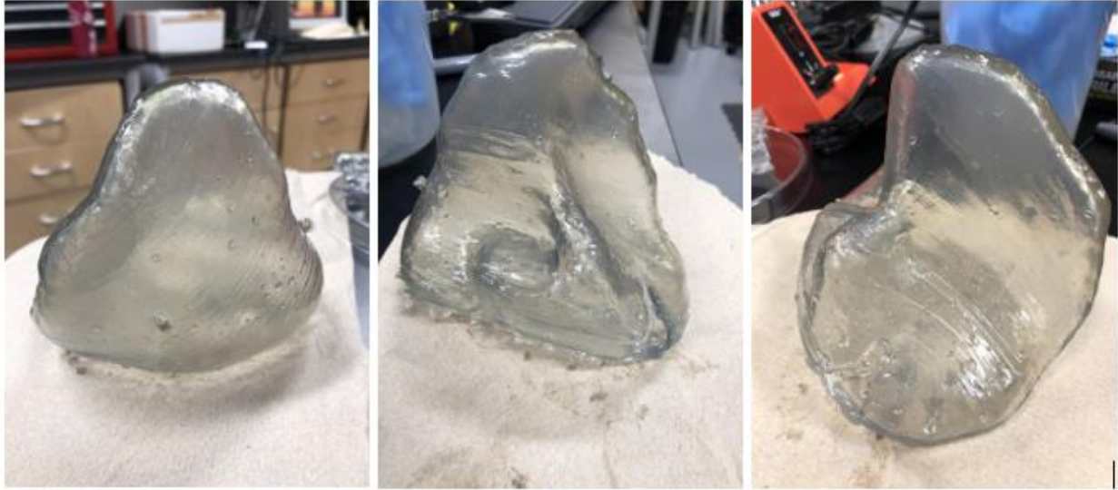
Figure 37. Final lung phantom print using custom resin formulation on custom designed SLA-DLP machine
