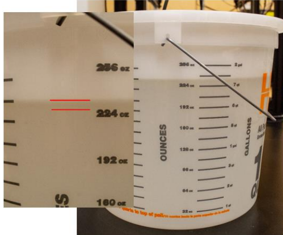
Figure 38. 10 qt. vat with suspended custom developed UV photopolymer resin suspended, marked in red
