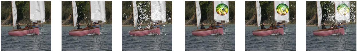
Figure 1.1: (From left to right) The original image with a label of yawl; masking its top 0.2% attribution; masking its top 4% of attribution; image with a banana adversarial patch [1]; masking its top 0.2% attribution; (rightmost) masking its top 4% of attribution. The classification result for the original image is robust and conforming in the neighborhood obtained by removing top positive attributions. The model predicts the original label (yawl) in the neighborhood. But the prediction changes from banana to yawl for many samples in the attribution neighborhood of the adversarial image. We observe a similar difference in conformance for the out-of-distribution examples and the adversarial examples generated by state-of-the-art digital attack methods such as DeepFool [2], PGD [3], FGSM [4] and Carlini-Wagner (CW) [5]. This observation motivates the use of conformance in the attribution-neighborhood as a confidence metric.
