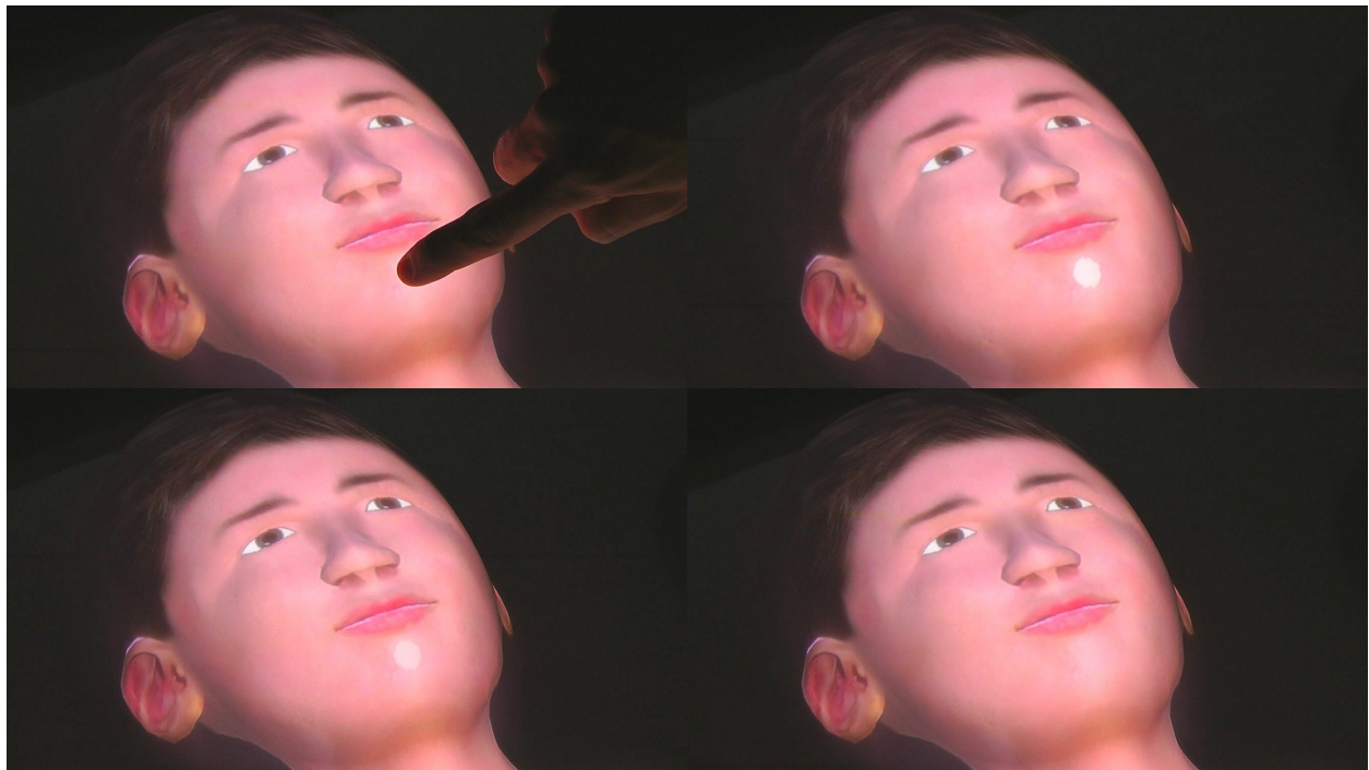
Figure 5.23: Touch-initiated capillary refill on the physical-virtual child surface, shown exaggerated for easier visibility. This interaction simulates the temporary restriction and subsequent return of blood flow at the point of contact. Time progresses from left to right and from top to bottom.
