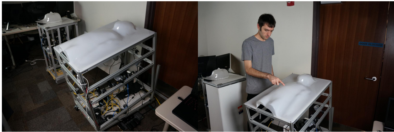
Figure 5.21: The touch-sensitive physical-virtual child surface.
