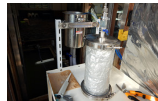
Fig.5 Hydrogen generation experiment equipment using acidic hot spring water and aluminum.
