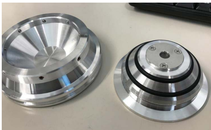
Figure 1. A target holder for irradiation of B 4 C-based ceramics
