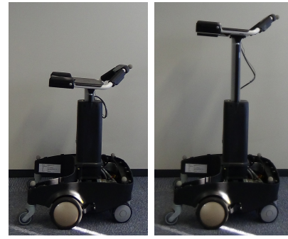
Fig. 5. Developed Assistive Robot (Left: Lowest Armrest, Right: Highest Armrest)
