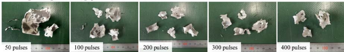
Fig. 10 Products obtained from the secondary crushing step of the back sheet layer.
