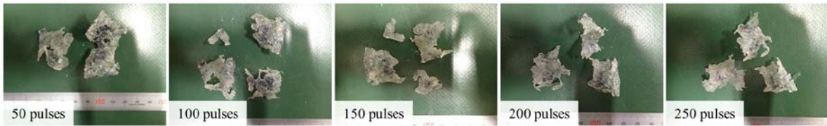
Fig. 4 Products obtained from the secondary crushing step of the glass layer. (glass particles were removed)
