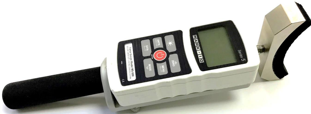
Figure 11. Digital force gauge and attachments
