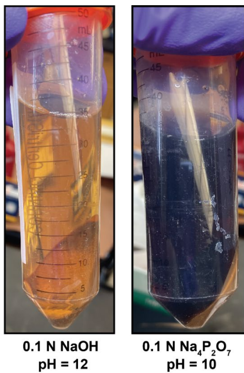
Figure II-1: Photographs comparing the NaOH and \text{Na}_4\text{P}_2\text{O}_7 organic matter extraction solutions.
