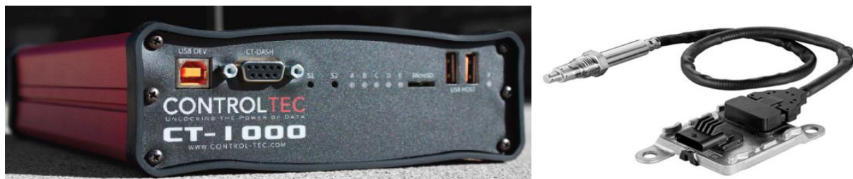
Figure 40: Picture of data acquisition hardware (a) Left image: PAMS (controltec) (left); (b) Right image: Continental Uni-NOx 2.8 tailpipe NOx sensor (right)
