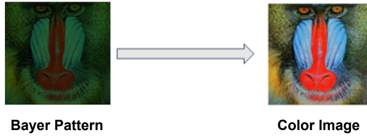
Figure 1.2: The general procedure of single image demosaicing.
