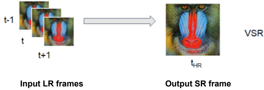
Figure 1.4: The general procedure of multi-frame video super-resolution.
