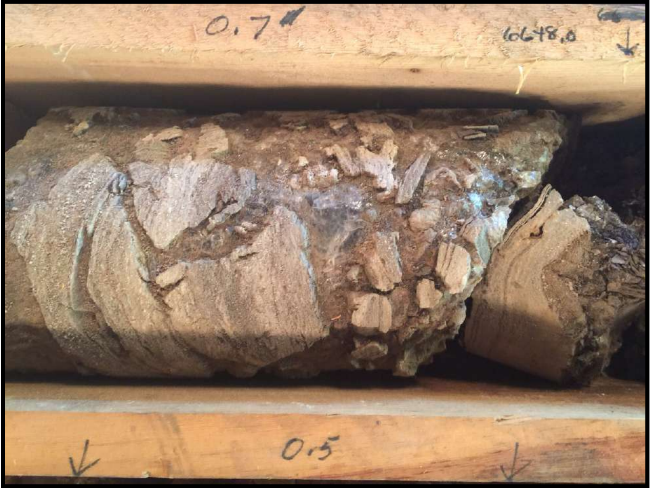
Figure 4-15. Mix of gray coarse crystalline halite as above and disoriented large (up to 0.8 ft) clasts of thin bedded anhydrite-carbonate plus calcareous shale. Core base is 6,648 ft.
