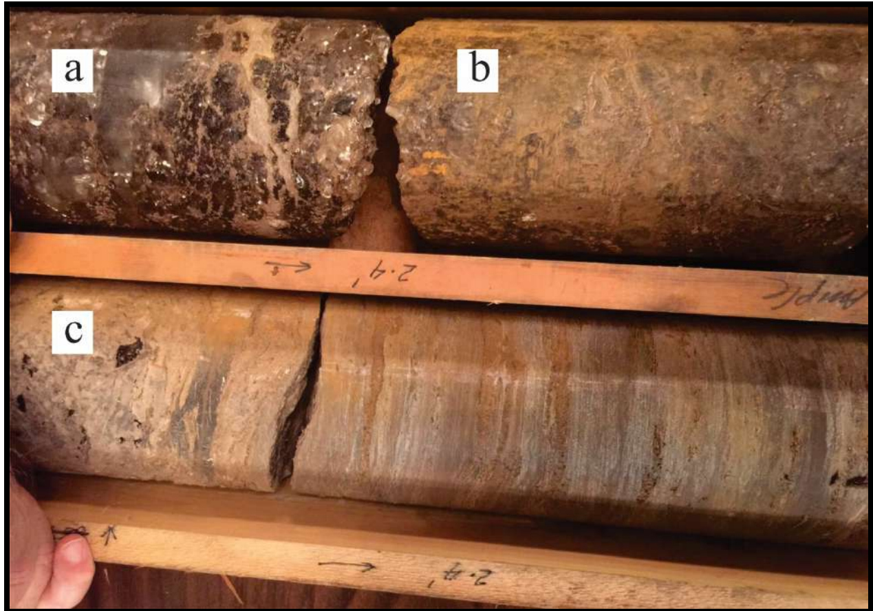
Figure 4-13. a: Coarse halite crystals with evenly disseminated black anhydrite pieces that give the sample a dark gray color; b: post-lithification fracture includes some salt crystals along the fracture zone; c: brown-gray calcareous shale, thinly laminated, sometimes wavy, partially replaced by salt and pepper carbonate(?) - anhydrite mixture. The shale is interbedded with the carbonate-anhydrite beds.
