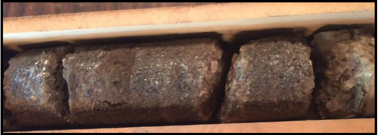
Figure 4-14. Uniformly coarse (0.25-0.5 inch [in]) halite crystals with evenly disseminated black anhydrite pieces, which give the sample a dark gray color.
