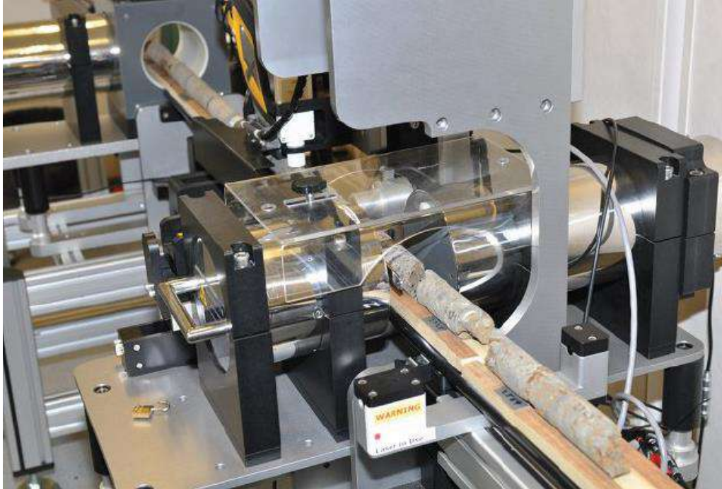
Figure 8-15. The GeoTek Multi-Sensor Core Logger (MSCL) scanning Lost River core at NETL. Photograph by Karl Jarvis.
