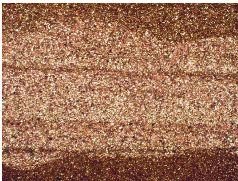
Figure 5-12. Thin section photomicrograph from the Richman Farms well showing ripple cross lamination overlying scour surface from Richman Farms well.
