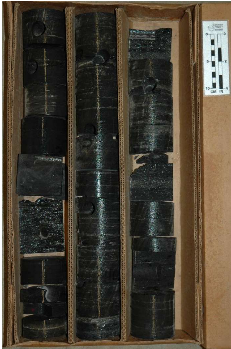
Figure 8-20. Photograph of the Point Pleasant interval in the Fred Barth No. 3 (API#3403122838), 5660-5670 ft. Note the significant number of plugged and slabbed segments.
