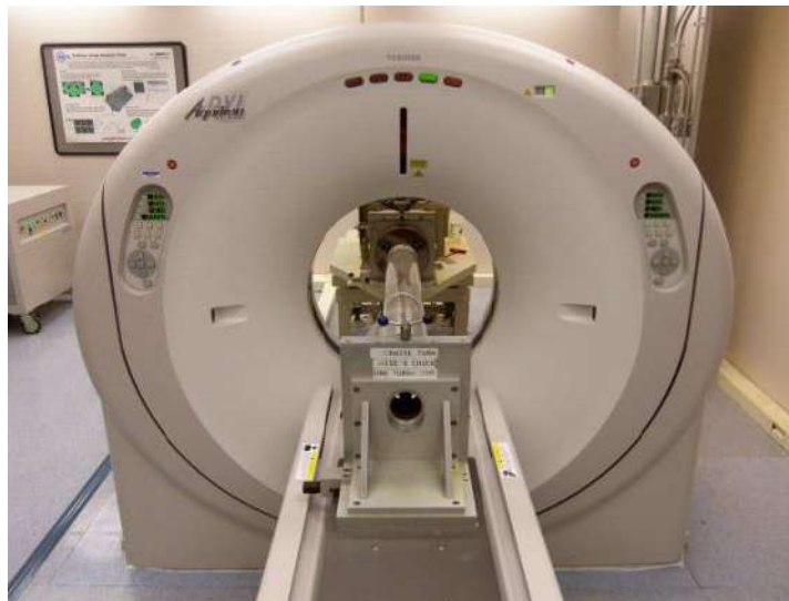
Figure 8-8. A 16-slice Aquillion medical CT scanner, similar to the unit in use at NETL.
