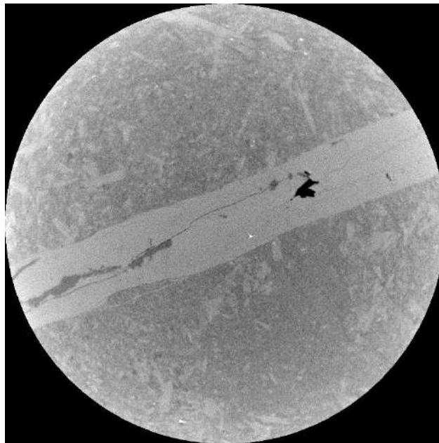
Figure 8-11. Scanned image of single layer of data along an XY plane through a one-in diameter sample of Marcellus Shale containing a mineralized fracture. Data obtained from the NETL industrial scanner.
