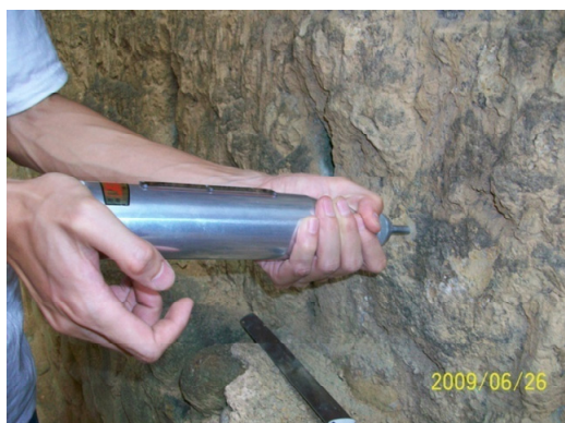
Figure 7. Rebound hammer being used to test the rammed earth wall.
