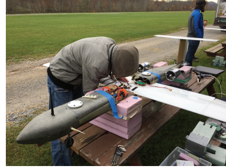
FIGURE 3: Phastball SUAV research platform. The two GNSS antennas are separated by an 85.3 cm baseline.
