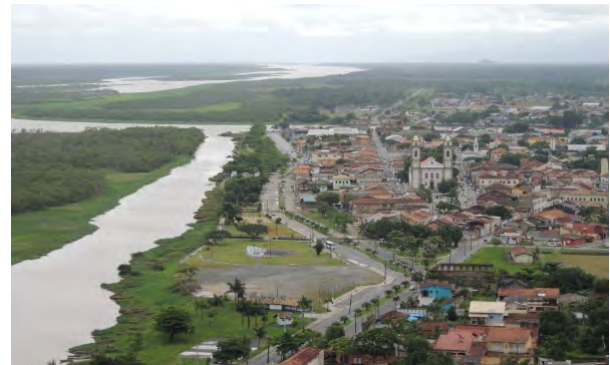
Figure 4: Islands formed at the mouth of the Valo Grande artificial channel, as a result of intense siltation in the area (Photo by Michel M Mahiques)
