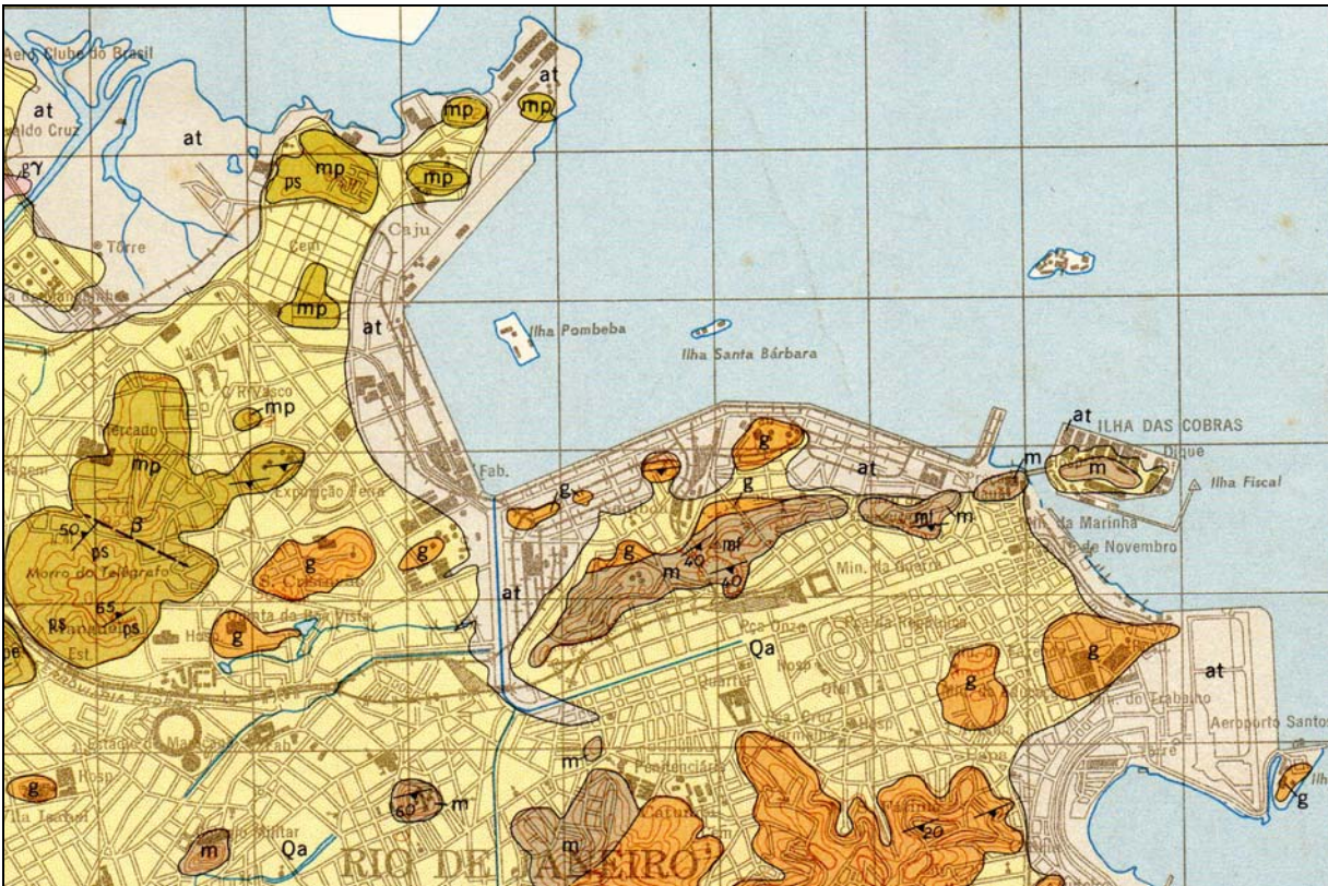
Figure 3: Technogenic land shape compartments: an extract of Guanabara State Geological Map, original scale 1:50.000 (Brazilian Ministry of Mines and Energy, Geology and Mineralogy Division, 1965). The “at” grayish areas near the shore are settings of flat lands (embankments) built up by technogenic deposits (made ground)
