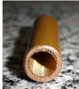
Figure 5. General view of the screen-covered groove capillary structure.
