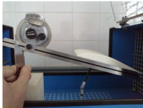
Figure 6. Method used to measure airfoil angles of attack (clockwise direction).
