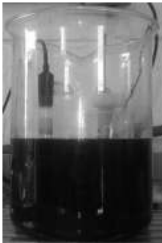
Figure 3. H_2SO_4 added to waste water from dyeing process (stage 1).
