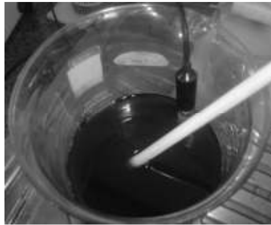
Figure 4. Coagulant – flocculant and decolourant added to the effluent (stages 2 and 3).
