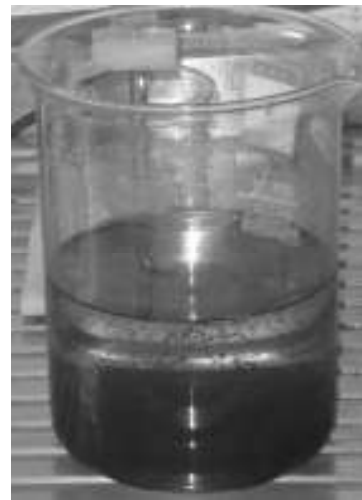
Figure 5. Amphoteric polymer added to the effluent (stage 4).
