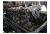
Figure 4. Rocker arm mounted in the motor.
