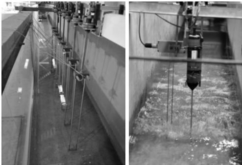
Figure 3. Eight wave gauge mobile structure (left) and the ADV probe with the wave gauge (right).
