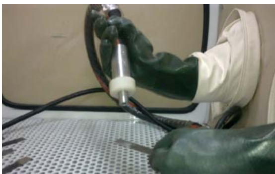
Figure 4. Blasting process with steel grit.
