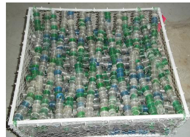
Figure 5. PET wire and Bottle necks.
