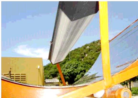
Figure 3. Absorber gutter in the system focus.
