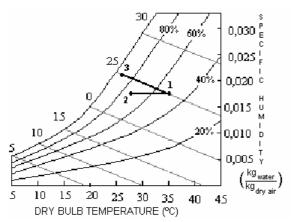
Figure 4. Psychometric chart showing the condition: (1) outside air, (2) air leaving the indirect unity and (3) air leaving the direct unity.
