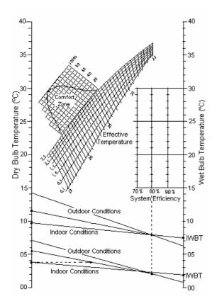
Figure 7. Nomograph and template (Camargo, 2000).
