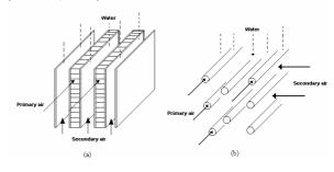
Figure 2. Indirect evaporative cooling: (a) type plate, (b) type tube.
