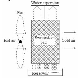
Figure 1. Direct evaporative cooling (DEC)
