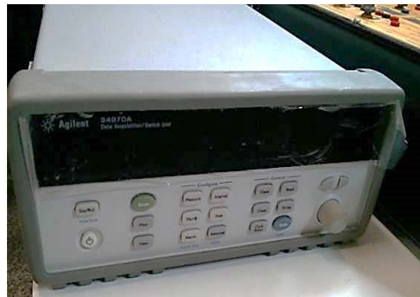
Figure 9. Data Acquisition Agilent 34970A.
