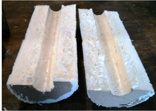
Figure 6. Thermal insulator constructed using polyurethane foam.
