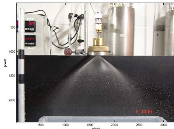
Figure 8. Not calibrated image of the cone angle measurement.
